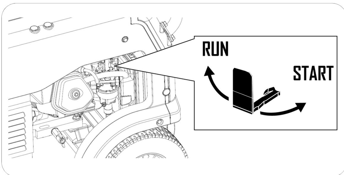
**Information:** If the engine has recently stopped and is still hot, the choke position procedure may not be necessary. In this case, to start directly, place it in the **RUN** position.
