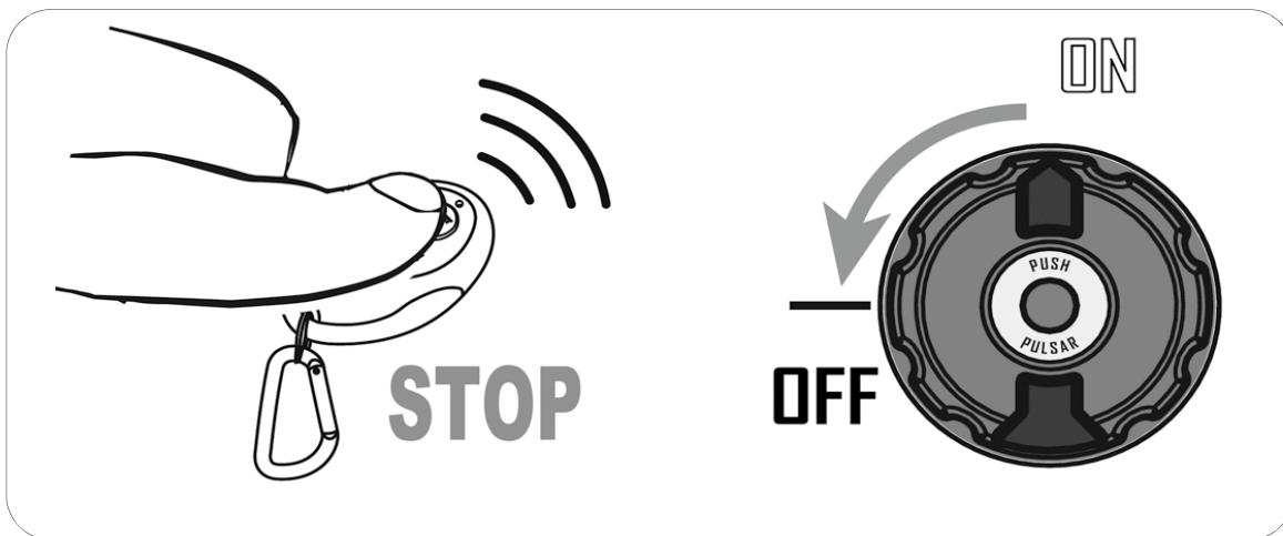
**NOTE:** Never, do not stop the automatic sequence of the starting or of the shutdown. Only in case of an emergency. The automatic sequence has to be finished, before to send a new signal from the remote control device.
