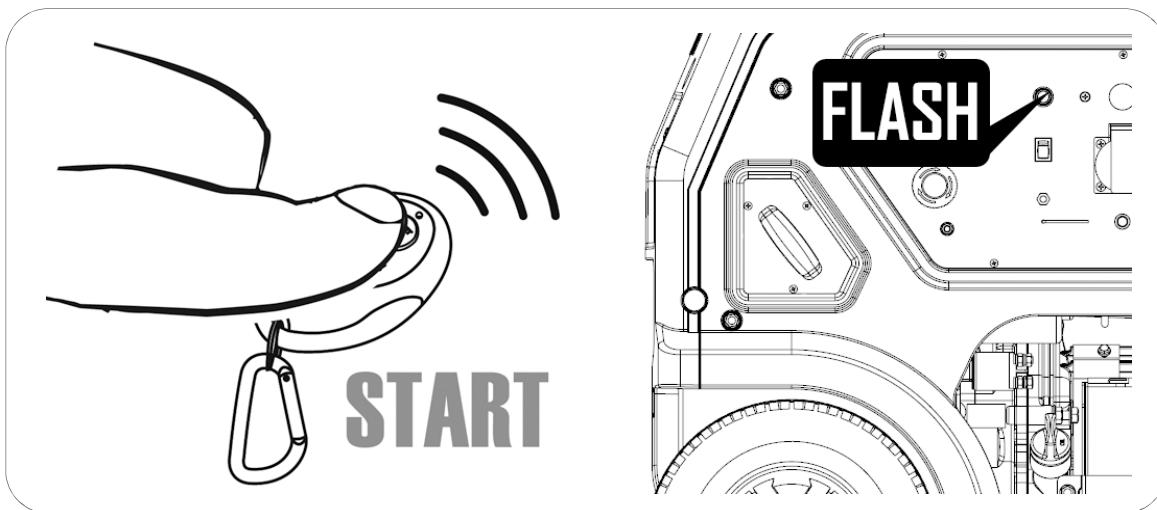
**Information: OPD Function** (Output power delayed). Up to 20 seconds after the starting, the generator does not generate electricity in the socket. This ensures that the generator starts without supplying power to the connected equipment.
