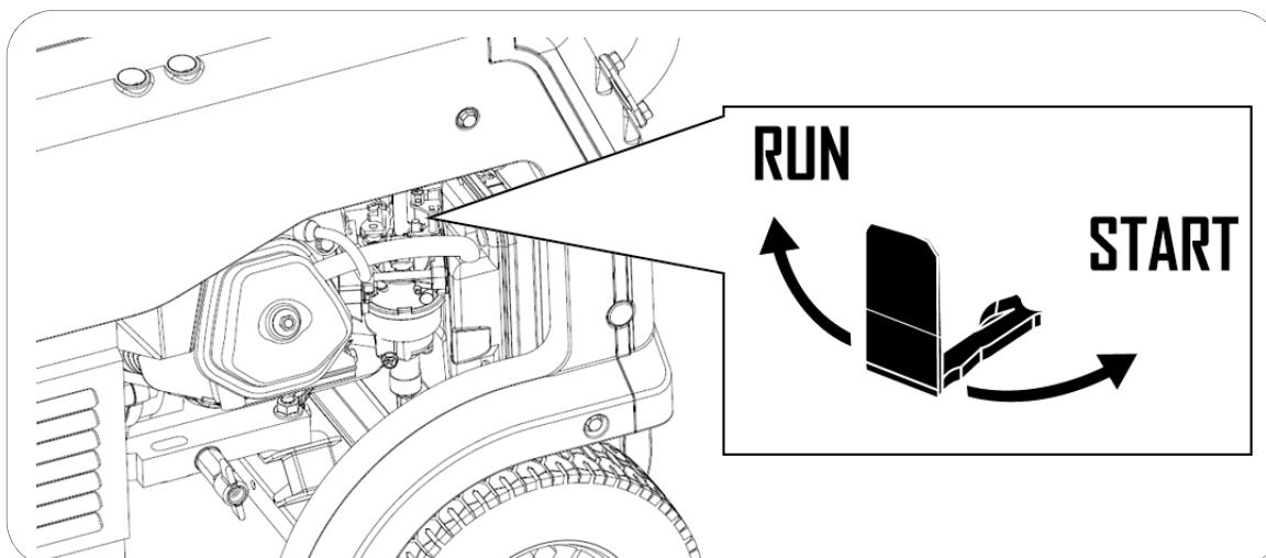
**NOTE:** The engine must not be kept running with choke in the **START** position, because the mixture would be too rich and cause engine problems. So as soon as the engine is started, the user must ensure that the choke is placed in the **RUN** position.
