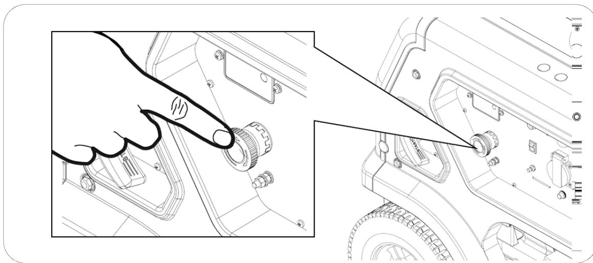
**NOTE:** Use the emergency stop button only when a dangerous situation occurs, otherwise, turn off the generator by the normal method.
