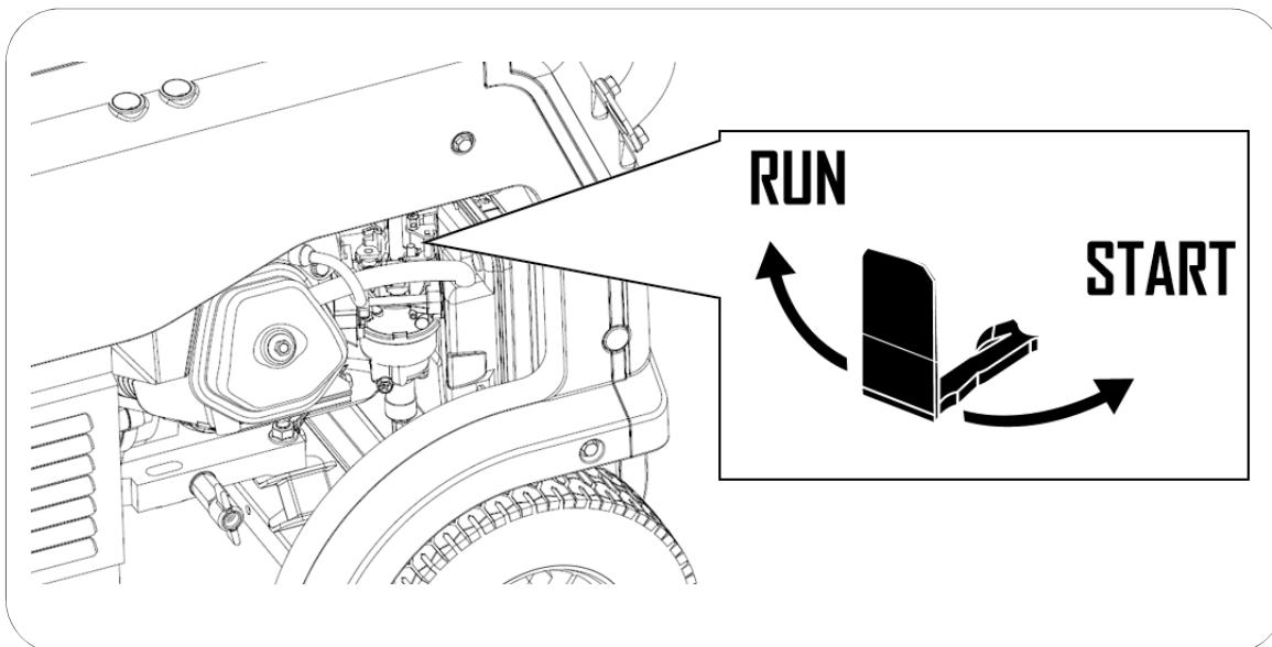
**Information:** If the engine has recently stopped and is still hot, the choke position procedure may not be necessary. In this case, to start directly, place it in the **RUN** position.
