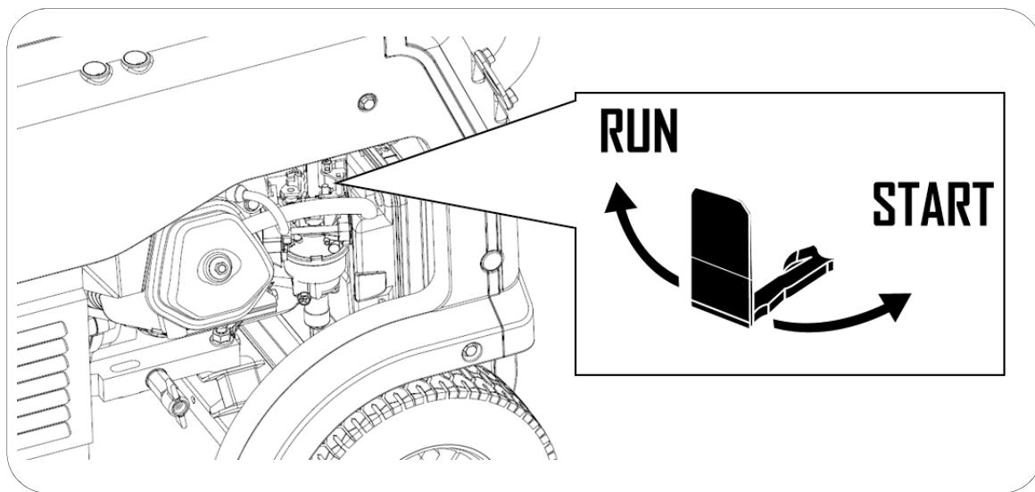
**NOTE:** The engine must not be kept running with choke in the **START** position, because the mixture would be too rich and cause engine problems. So as soon as the engine is started, the user must ensure that the choke is placed in the **RUN** position.
