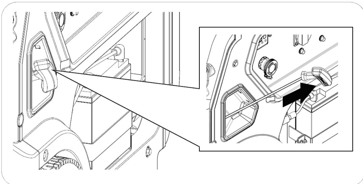
**NOTE:** If the rope recoils abruptly, the spring or the rope itself may be damaged. This is not covered by the warranty.
