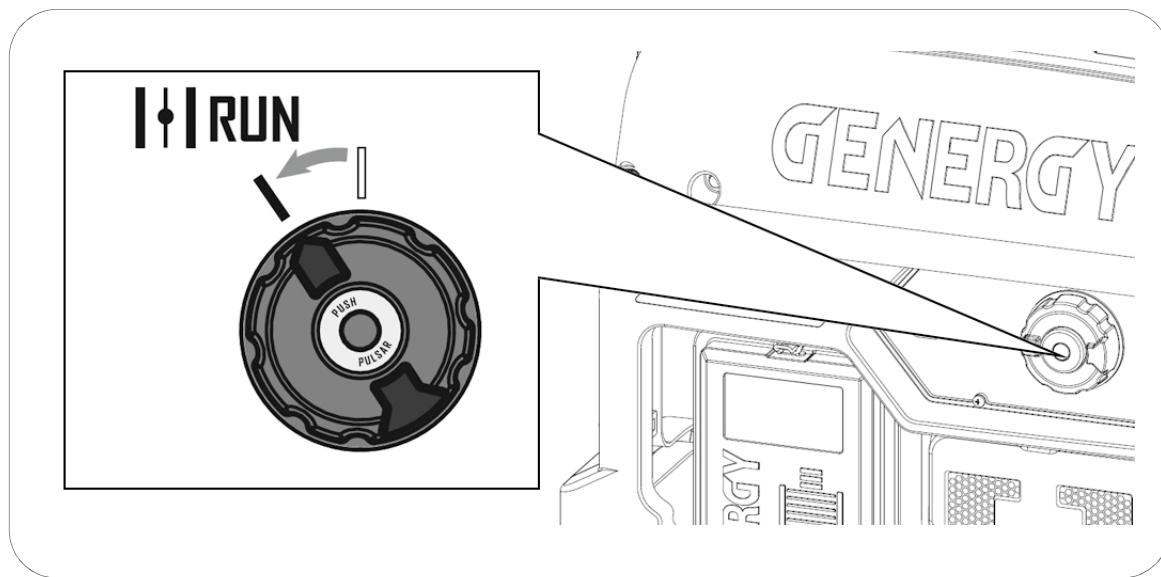
**NOTE:** The engine must not be kept running in the **CHOKE** position, because the mixture would be too rich and cause engine problems. So as soon as the engine has started, the user must ensure that the DIAL is placed in the **RUN** position.
