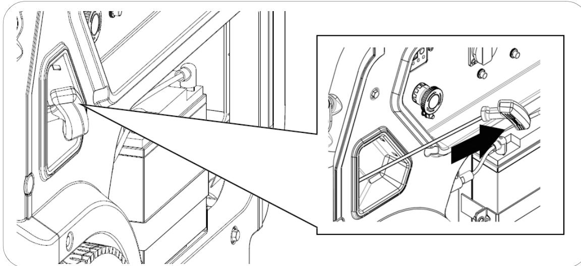
**NOTE:** If the rope recoils abruptly, the spring or the rope itself may be damaged. This is not covered by the warranty.
